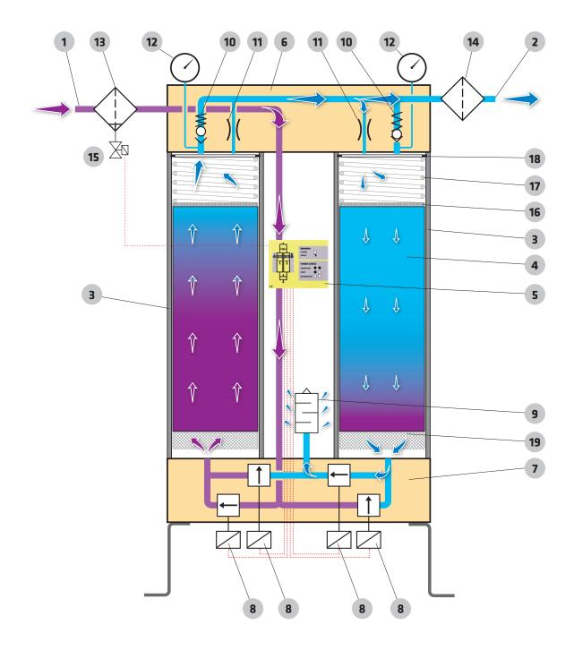
A-DRY adsorption dryers have been designed for continuous separation of water vapour from the compressed air thus reducing the pressure dew point.
